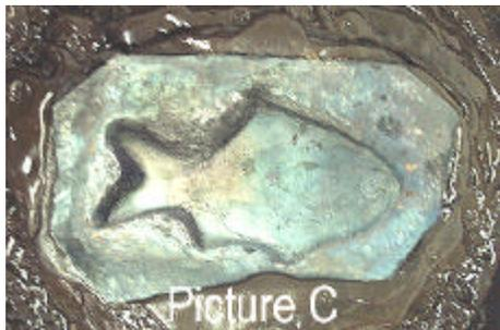
Turn the metal upside down and fill it with small pieces of pitch like before. Carefully heat it and put it back into the pitch pot. Take the hammer peen and begin making a trench about an inch and a half out from the edge of the pattern. Work towards the wall of the pattern raising it a little higher.
