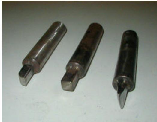
The butcher will make a clean separation between what is to be drawn out and what is not, without a lot of errant hammer marks screwing up the transition. I use it on set downs, like the light switch plate I did at the meeting.
