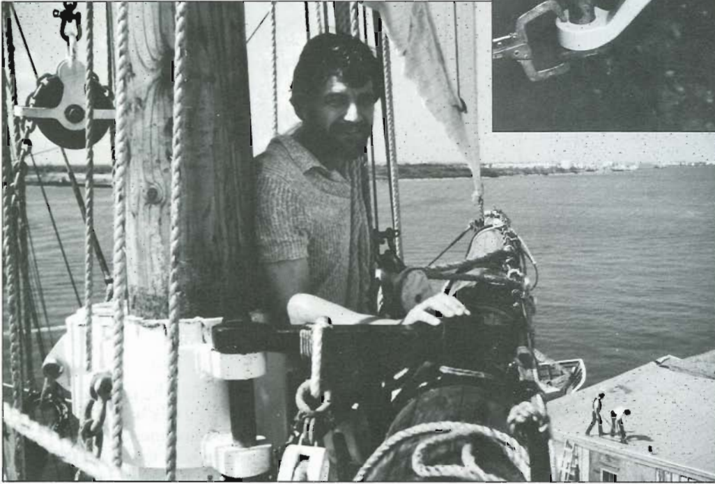
Lower topsail yard crane installed.
