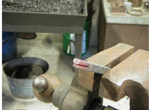
At this point you should have a bar with one end split leaving 3 pieces. The two 1/4" wide pieces of the split will form the wings and the 1/2" part will form the body and tail.
