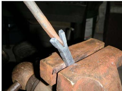
Place in a vise and use the hot cut chisel to make the cut square at the bottom.
