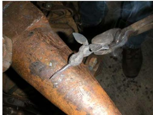
Heat and form the beak. Forming the beak is the hardest part of forging a Hummingbird. If you are not careful, you will either crack or break off the beak.
